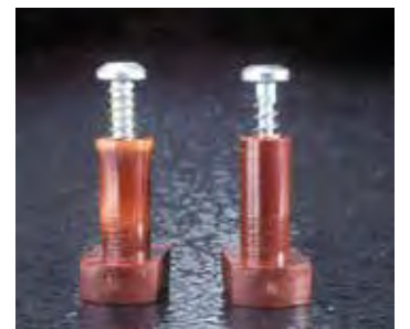
Too much thread engagement can result in increased radial stress (left image)
