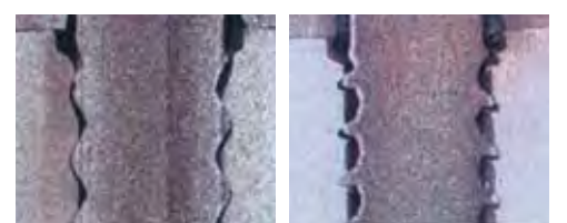
Since Mag-Form screws (left) use a compressive force to create threads in magnesium, the result is close-bonding threads. A thread-cutter of the same size requires a larger hole for chips, so the thread engagement is much lower.
