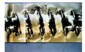
In plastics, incorrect hole size and/or installation torque can result in damaged holes.
