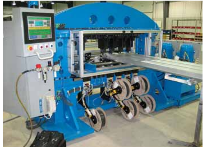
Self-pierce riveting equipment is available in a wide variety of configurations. Here, five rivet setters are grouped together in an H-frame. A servo-driven indexer moves parts into the system.
