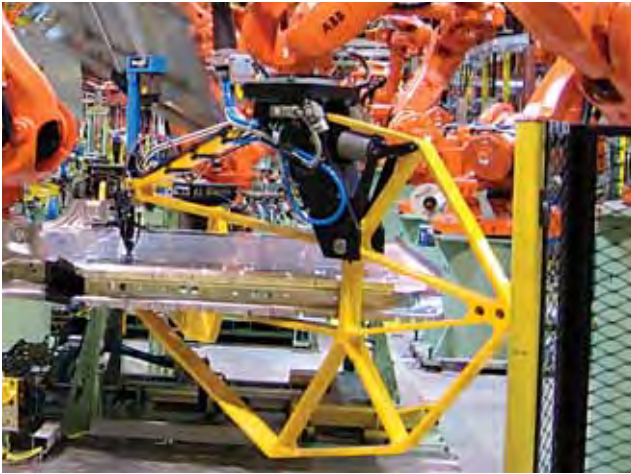
Freightliner uses self-pierce rivets to assemble aluminum parts for its new Class 8 Cascadia truck. Here, a six-axis robot moves a lightweight C-frame to rivet a floor assembly. The C-frame allows the riveter to access areas more than 4 feet into the assembly.
